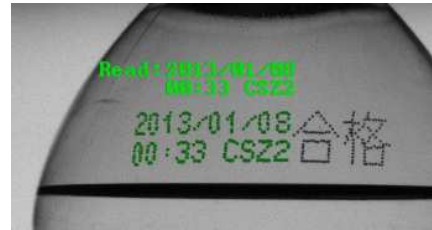
Result of data extraction using OCR.
