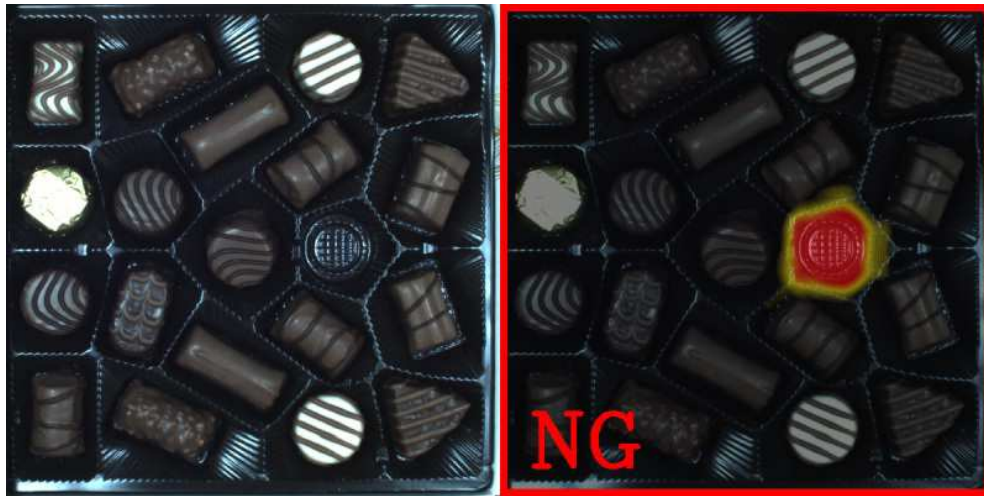
An example of a missing object detection using FisFilter_DL_DetectAnomalies2 tool. Left: The original image with a missing element. Right: The classification result with a heatmap of anomalies.
