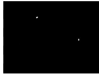
Result of thresholding reveals the location of the red dots on the globe.
