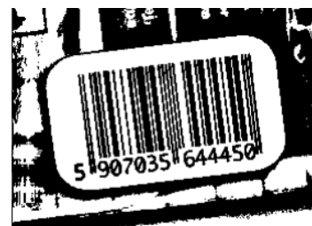
Result of ThresholdImage_Dynamic – the bars are correct.
